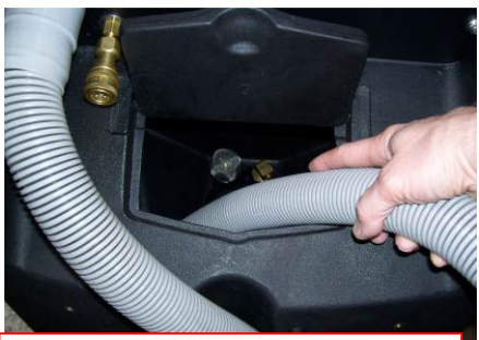
Vacuum acid solution out of Solution Tank
