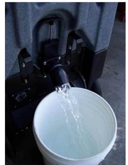
Draining the Recovery Tank
