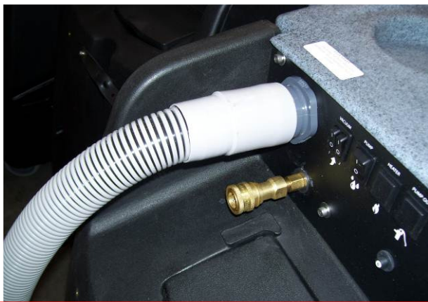
Vacuum Hose connection with standard barb and vinyl cuff
