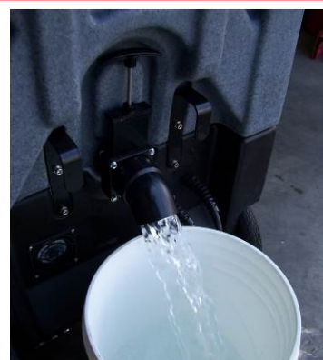
Drain water from Recovery Tank
