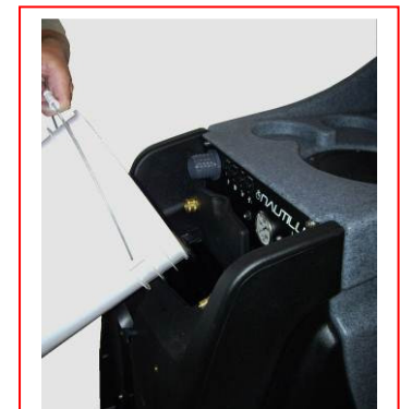
Pour 2 or 3 gallons of clean water into Solution Tank
